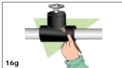
Follow the procedure for the insulation of flanges as previously illustrated using a sheet of insulating material.
