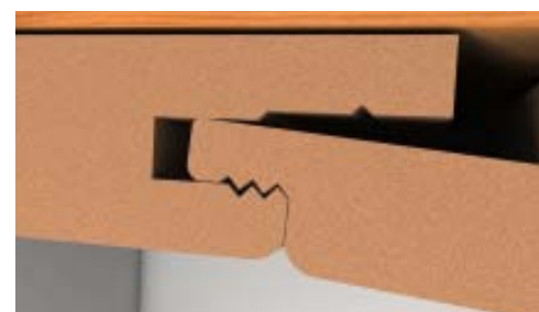
The innovative click mechanism effectively prevents the mounted panel from sliding out.
