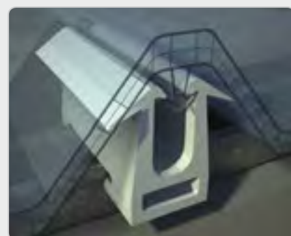
ANCHORAGE OF ROOFING This is done by pressing onto the anchor bracket
