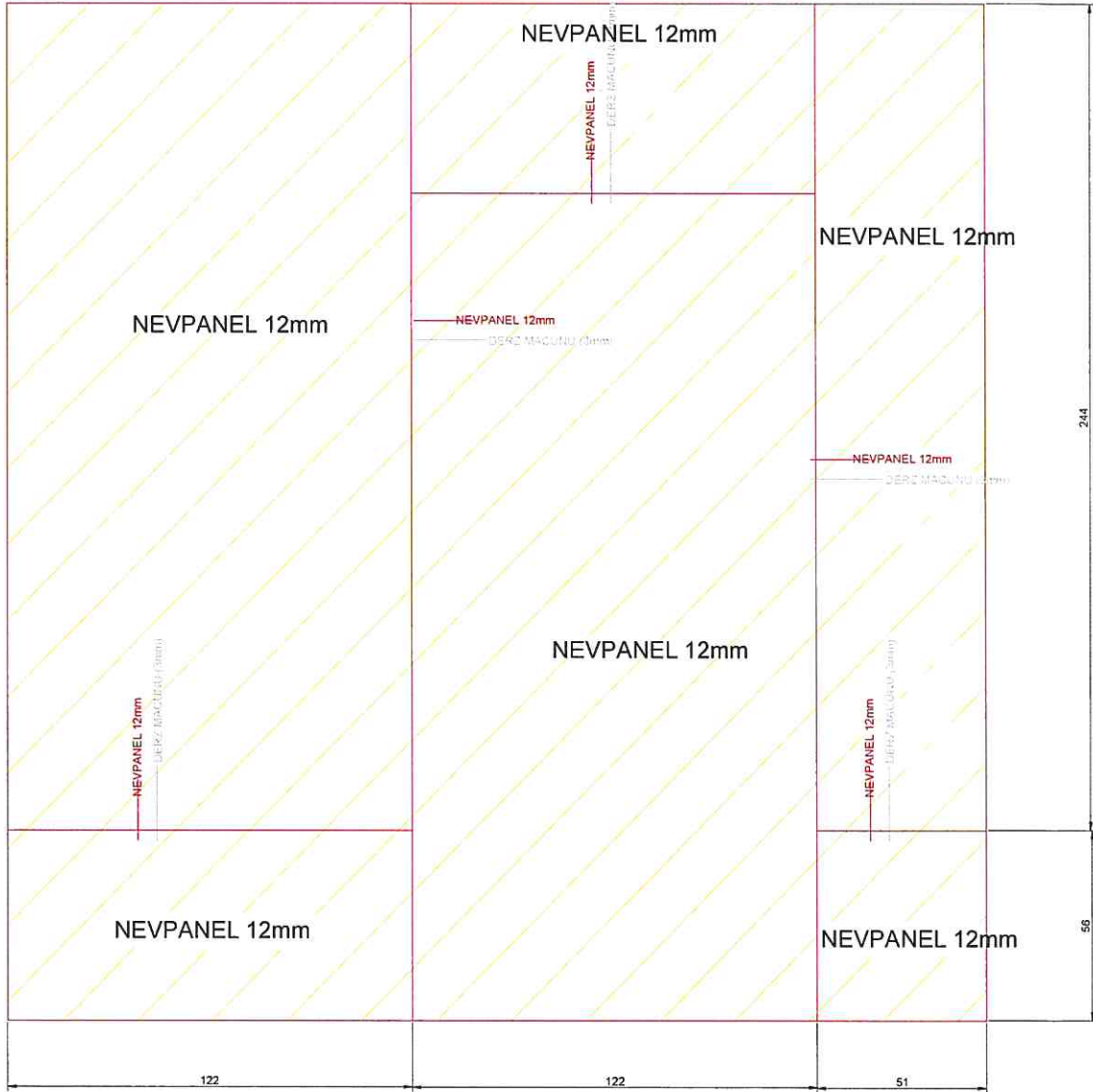
Figure 6: Details of 3. layer panels
