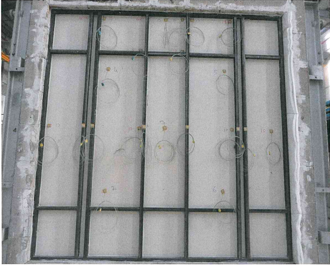
Photo C1: Unexposed side of the test specimen before the test
