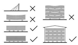
Valchromat panels must be stored in a covered area, protected from sunlight and rain, with a flat and horizontal base. The pallets must be placed on supports with sufficient height (≥8 cm) to allow easy access with a forklift. The maximum distance between supports should not exceed 800 mm.
