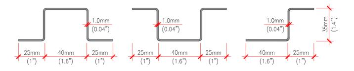
Figure 2.20 - Section type of structure in galvanized steel DX51D (Z+) (Dx51D Z+ galvanized steel)
