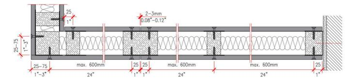
Figure 2.16 - Horizontal section of the wall, wooden structure
