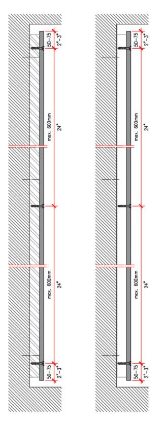
Figure 2.23 - Vertical section Wooden structure and galvanized steel
