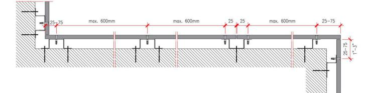
Figure 2.22 - Horizontal section, galvanized steel structure
