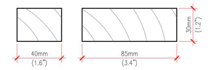
Figure 2.19 - Section type of wooden structure (Class C18 Resistance)
