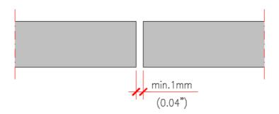
Figure 4.8 - Joint between panels
