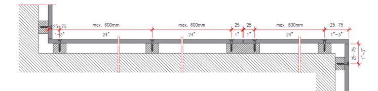
Figure 2.21 - Horizontal section, wooden structure
