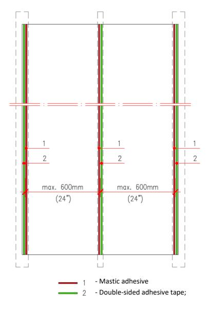
Figure 2.2 - Gluing system location
