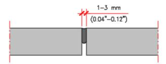
Figure 3.14 - Joints between panels with mastic
