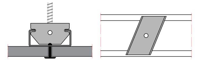
Figure 4.6 - Panel attachment detail to the support section
