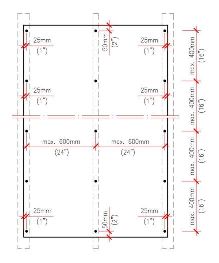
Figure 2.8 - Nail location (Distances to the edges and between elements)
