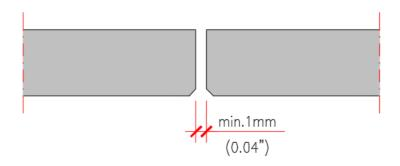
Figure 4.9 – Bevelled edge
