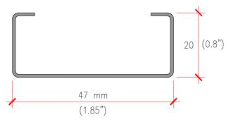
Figure 4.4 - C profile, galvanized steel Dx51D (Z+)
