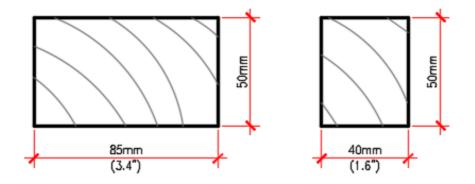
Figure 2.12 - Section type of wooden structure (Class C18 Resistance)
