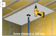
Forestia Premium Ceiling panels are screwed into the groove with a wooden screw. Use a lowering head 3.0/35mm or equivalent. Screw distance must be 150 mm. A stapler can also be used. They should have a straight back, min. a width of 10 mm and the length of the legs should be min. 35 mm. **NB!** Pressure on the staple gun must be adjusted carefully. Staples/screws must not be submerged, but must follow the surface in the grooves.
