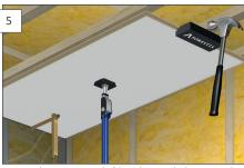
Use a ceiling support to hold up the panels during instal lation. The Forestia tapping block must be used to avoid damaging the profile when the panel is to be clicked into place. This tapping block is adapted to the panel's profile.
