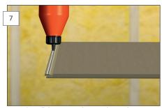
Cut and install the next panel. Remember to glue the short-end profile. We recommend PVAc glue or equivalent.
